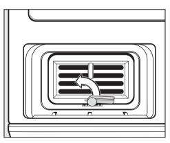
Turn the lever on the condenser unit to the vertical position so that the hook on the lever is no longer in the groove at the bottom of the condenser unit housing.
